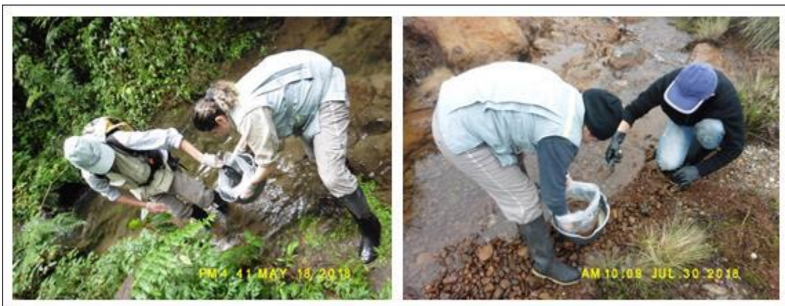
Figure A3.3.9. Sampling of stream and suspended sediments for the determination of arsenic and other potentially harmful elements.
