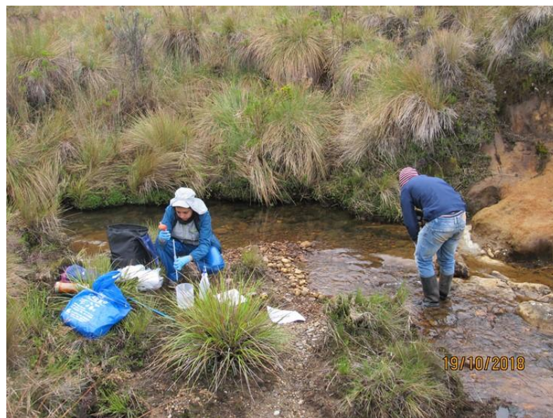
Figure A3.1.4. Collection of water samples for arsenic evaluation in waters of water basins of Risaralda, Colombia. Photograph belonging to the SGC archive.
