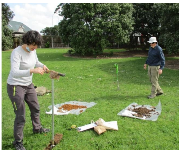
Figure A3.18. Collecting soil samples from 3 depths during the urban geochemical soil baseline survey, Auckland, New Zealand.
